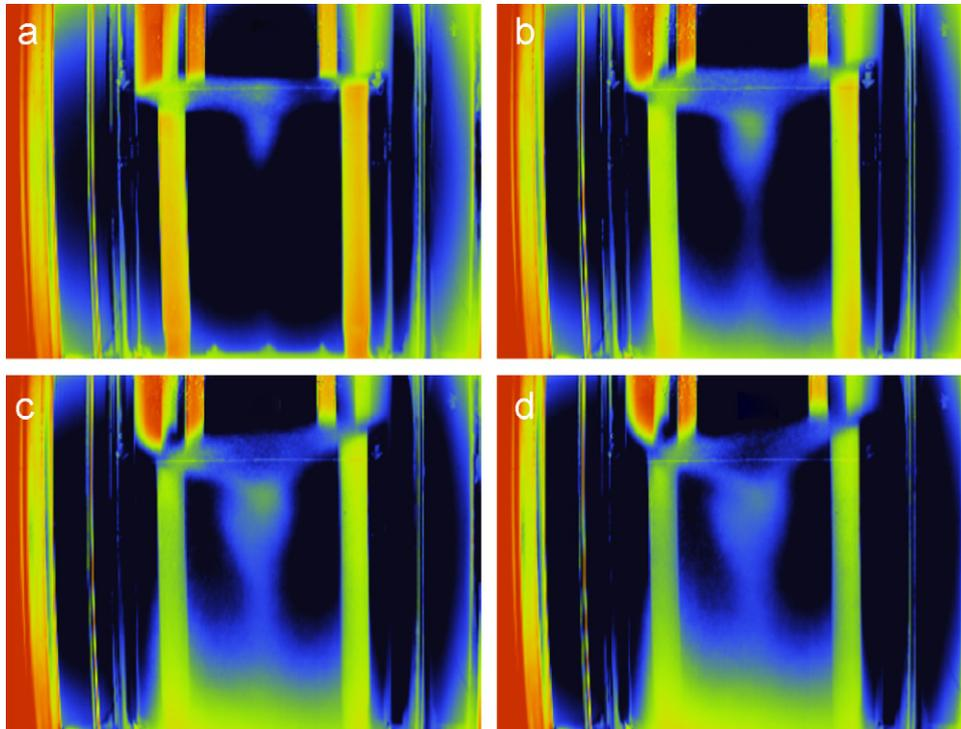
Fig. 11. Experimental acquisitions of the vortex shapes, negative coloured pictures: (a)  $N = 200$  RPM,  $G = 26,000$ ; (b)  $N = 250$  RPM,  $G = 22,500$ ; (c)  $N = 300$  RPM,  $G = 20,000$ ; (d)  $N = 350$  RPM,  $G = 18,000$ .
