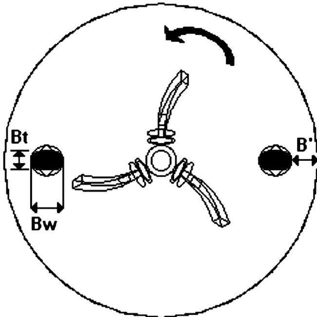
Fig. 3. Plan view of the mixing vessel.
