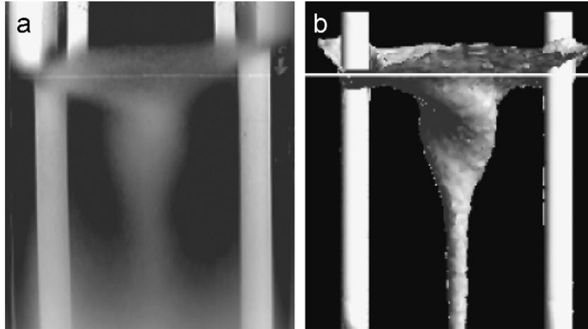
Fig. 10. Comparison on the same scale of the experimental (a) and the numerical (b) vortex shapes; (a) negative coloured picture,  $G = 21,000$ ,  $N = 275$  RPM and (b) isosurface of water volume fraction equal to 0.9 ( $N = 275$  RPM).
