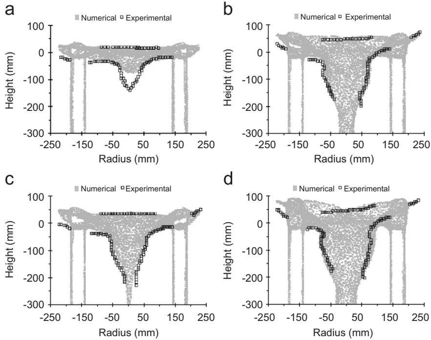
Fig. 12. Comparison between experimental vortex shapes (negative coloured pictures with the optimal gain) and the projection on the  $XY$  vertical plane of isosurfaces of water volume fraction equal to 0.9: (a) 200 RPM; (b) 250 RPM; (c) 300 RPM and (d) 350 RPM.
