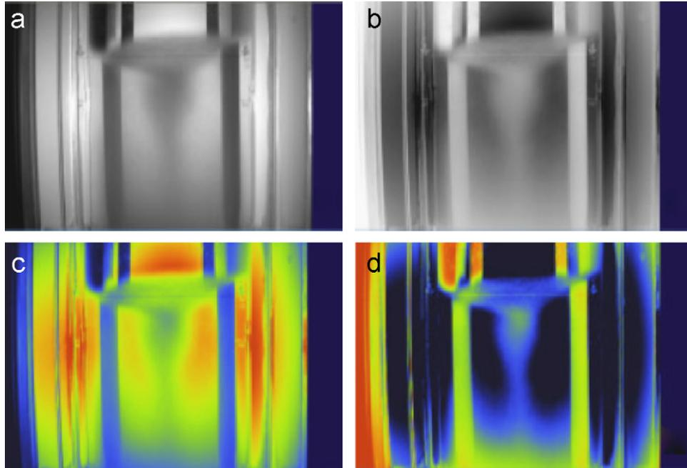
Fig. 5. Final vortex pictures,  $N = 275$  RPM. (a) Black and white raw picture; (b) black and white negative picture; (c) coloured picture by transformation of the grey levels of (a) and (d) negative coloured picture from (c) with  $G = 21,000$ .
