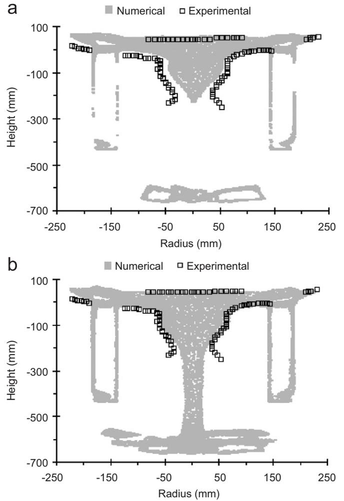
Fig. 9. Comparison between experimental vortex shape profile (negative coloured picture,  $G = 21,000$ ,  $N = 275$  RPM) and the projection on the  $XY$  vertical plane of isosurfaces of water volume fraction ( $N = 275$  RPM); (a) isosurface of water volume fraction equal to 0.5 and (b) isosurface of water volume fraction equal to 0.9.
