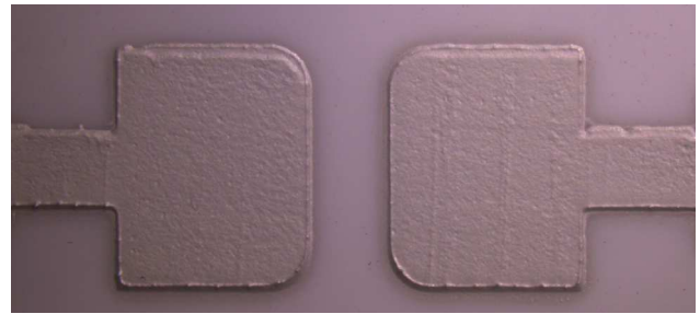
Figure 15: Image of the screen-printed silver electrodes after sintering, with a 2 mm gap.
