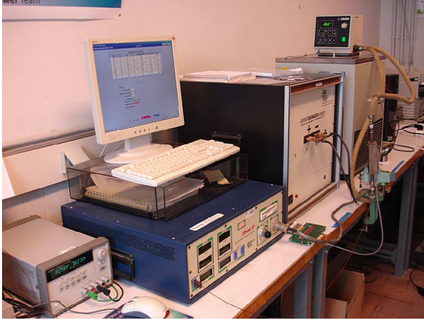
Figure 2 : test bench for thermal resistance measurement
