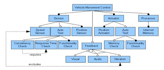
Figure 1: example of a simplistic vehicle movement control systems product line.
