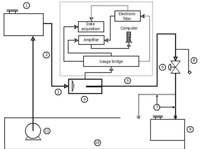
Figure 3: Sketch of the test loop.
