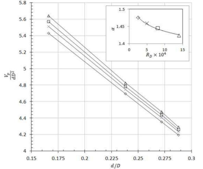
Figure 7: Variation of the dimensionless digital volume with confinements for several Reynolds numbers ( $Re_D$ ). Inset: parameter  $\alpha$  vs.  $Re_D$ , where the parameter  $\alpha$  is obtained by a fit of the form  $\frac{V_p}{dD^2} = V_r(Re_D) \cdot (1 - \alpha \frac{d}{D})$ .
