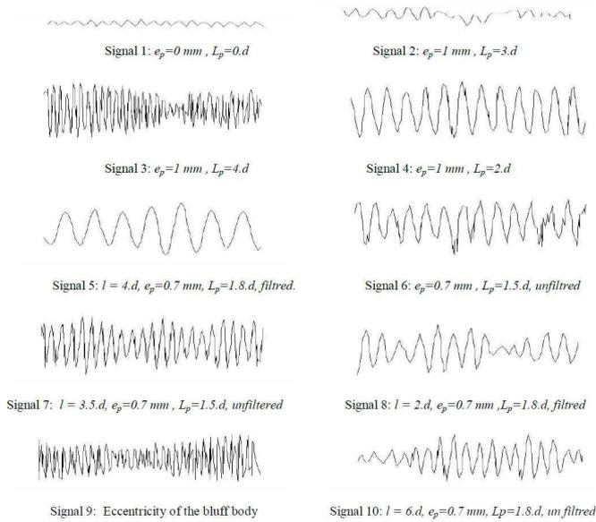
Figure 4: Representative Signals of the shedding vortices frequency.
