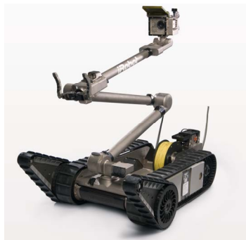
Figure 1. Morphology of an UGV (iRobot® 510 PackBot®). This small ROV (88.9 × 52.1 × 17.8 cm; 10.89 kg without batteries) can be used on a great variety of terrain (image courtesy iRobot®).
