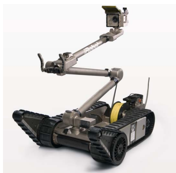
Figure 1. Morphology of an UGV (iRobot® 510 PackBot®). This small ROV (88.9 × 52.1 × 17.8 cm; 10.89 kg without batteries) can be used on a great variety of terrain (image courtesy iRobot®).
