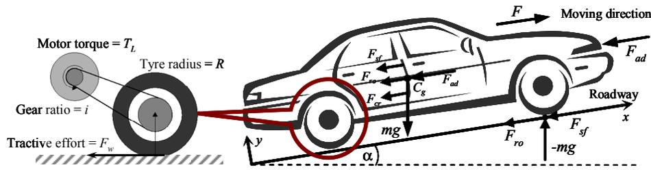
Fig. 4. Elementary forces acting on a vehicle.
