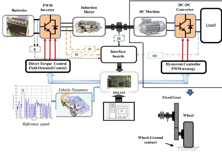
Fig. 2. EV HIL simulation platform.
