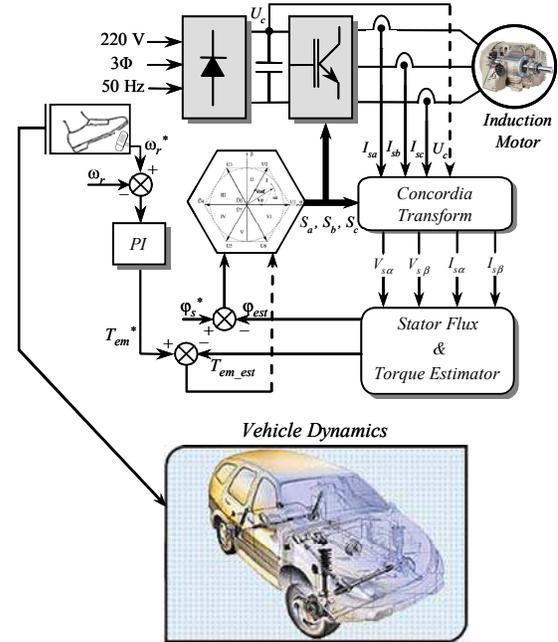
Fig. 3. DTC general configuration.
