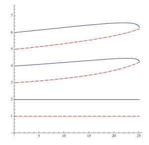
FIGURE 1. Using a shooting method, one can numerically compute the lowest eigenvalues of  $-\mathcal{L}$  for k = 0 (radial functions) and for the k = 1 component of the spherical harmonics decomposition (dashed curve). The plot shows that 1 and 2 are the lowest eigenvalues, when mass varies between 0 and  $8\pi \approx 25.1327$ . See [13] for details and further numerical results.
