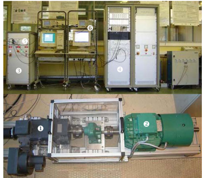
Fig. 17. Components of the G2Elab test bench, Grenoble, France: ① dc motor, ② DFIG, ③ Power electronics for driving the dc motor, ④ Power electronics for driving the DFIG, ⑤ DSP TMS320F240 implementing dc motor control, ⑥ DSP DS1005 (dSPACE) implementing PMSG-based MCT control.
