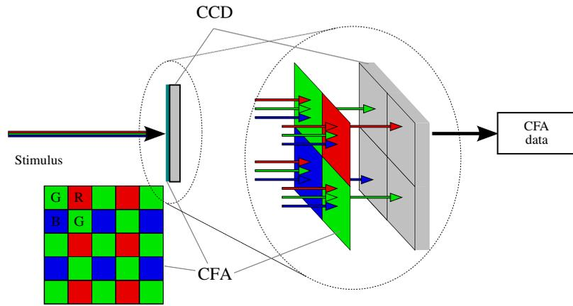
(a) Single-CCD technology (simplified), with filters arrangement according to the Bayer CFA
