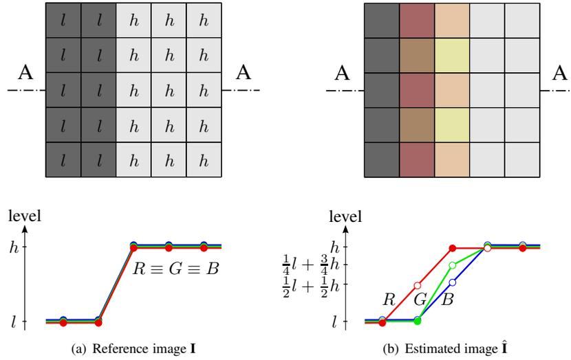
**Figure 6.6.** Marginal images and profiles of levels of pixels located on the center line A-A, for a reference image (a) and the corresponding image estimated by bilinear interpolation (b). In the profiles, the color dots denote available levels and the white dots denote estimated levels
