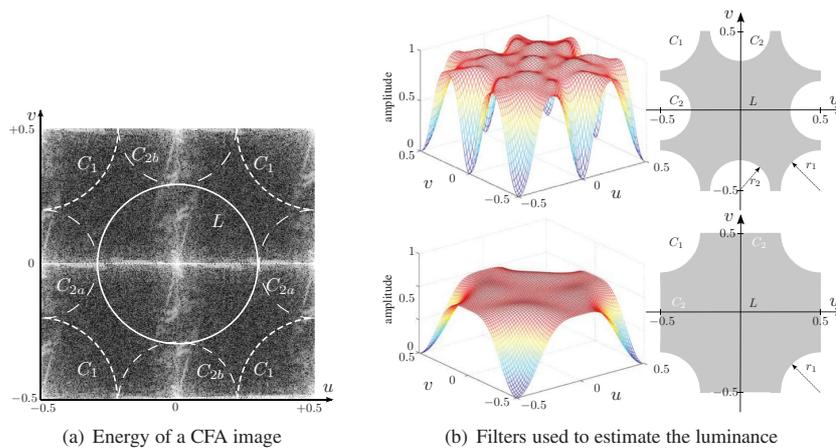
**Figure 6.8.** Frequency analysis of a CFA image (frequencies in cycles/pixel).
