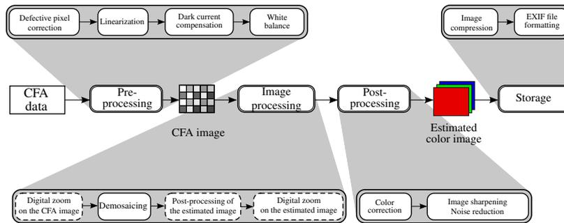
(b) Image acquisition in a single-CCD color camera (detailed diagram). Dotted steps are optional
