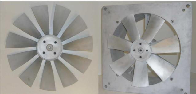
FIG. 2. Picture of the front rotor (left) and Rear Rotor (right)
