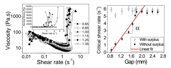
Figure 10: (a) Apparent viscosity and normal stress as a function of shear rate for different gaps in mm. Measurements were made with a parallel plate rheometer (Bohlin C-VOR 200) with radius R = 20 mm. (b) Evolution of the critical shear rate a function of the gap. The error bars correspond to the uncertainty (reproducibility) of the experiments.
