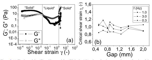
Figure 7: (a) Elastic modulus (G') and loss modulus (G") in the 44% volume fraction suspension as a function of shear strain for an imposed shear stress (0.001 to 100 Pa) at 1 Hz in a vane geometry. (b) Critical strain vs. gap and frequency
