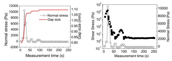
Figure 8: Time evolution for a  $\dot{\gamma} = 1.6s^{-1}$  applied shear rate of: (a) the gap size and the normal stress; (b) Normal (circles) and shear stresses (squares). The rheometer is set to change the rotation rate of the tool through a feedback loop to make sure the shear rate is constant, even though the gap is changing.
