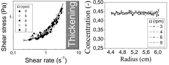
Figure 4: (a) Local shear stress as a function the local shear rate. The line is a fit to the Bingham model:  $\sigma = \sigma_y + k\dot{\gamma}$  with  $\sigma_y \approx 0.35 Pa$ , k = 0.30 Pa.s. b) Local concentration profiles in the Couette gap geometry for a cornstarch suspension sheared at various rotational velocities ranging from 3 to 9 rpm.
