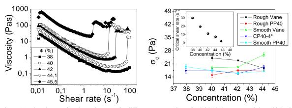
Figure 11: Viscosity as a function a shear rate for different concentrations. (b) Critical shear stress of shear thickening vs. concentration in different measurement geometries. Inset: Critical shear rate of shear thickening vs. concentration.
