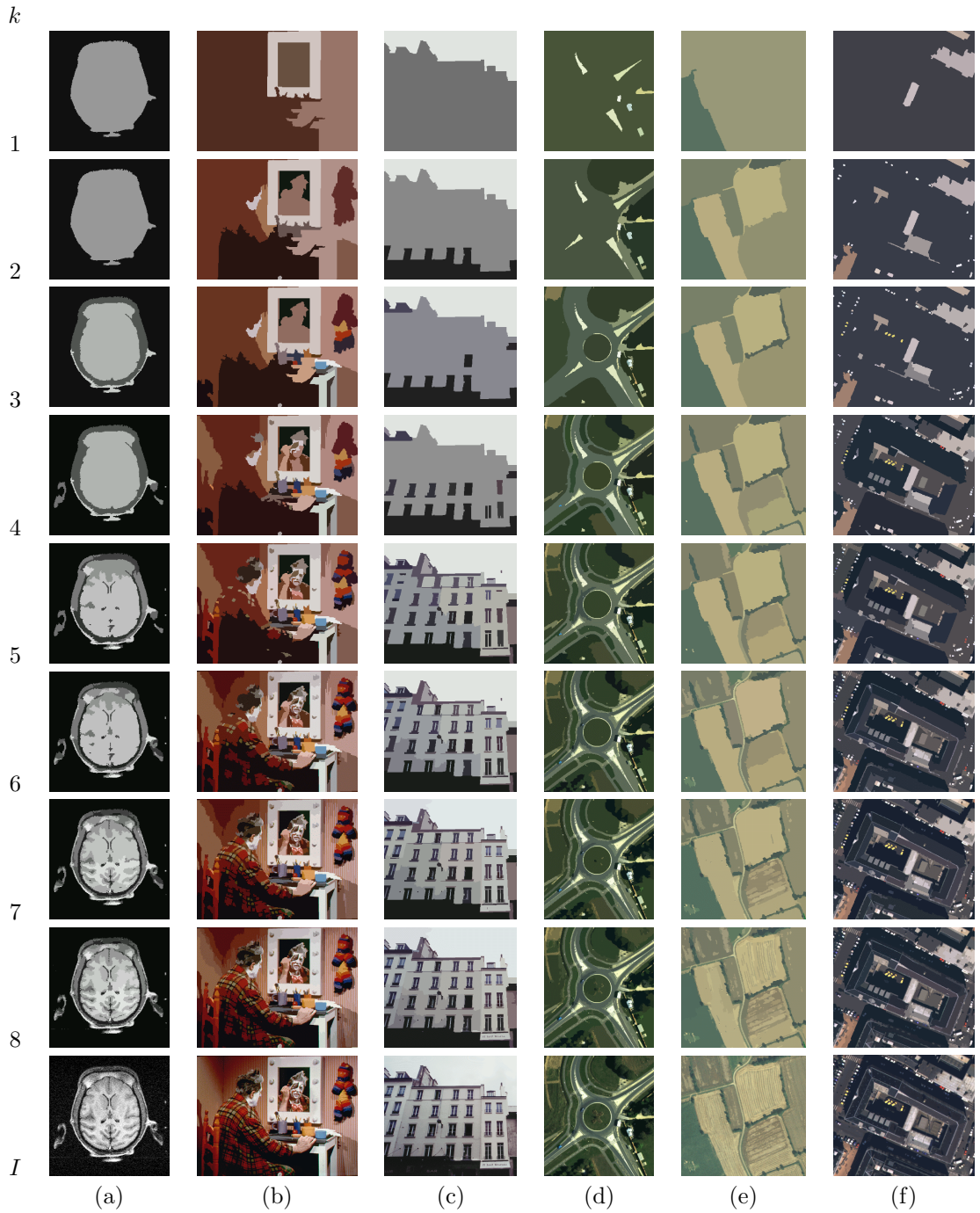
Figure 7: Dichotomies of some scale-sets obtained by scale climbing from the image pixels using Mumford-Shah's piece-wise constant model. k is the order of the dichotomy (see text). The bottom row represents the original images.
