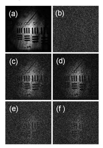
Fig. 9. (a,c,d): Reconstructions of an USAF target with different level of illumination 700 (a), 1 (c) and 0.15 e/pixel (d). (b): Simulated Shot Noise noise image. (e,f): Simulated reconstructed image obtained by mixing image (a) with weight X, and image (b) with weight 1 - X. The weight X is 1/700 (e), and 0.15/700 (f). Images are displayed in arbitrary logarithmic grey scale.
