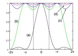
Fig. 7. One dimension (1D) angular response of the detection efficiency for the intensity  $\sum_m |\operatorname{sinc}(X + m\pi)|^2$  as a function of X for the main lobe: m = 0 (a); for the main lobe and 2 aliases:  $m = 0, \pm 1$  (b); for the main lobe and 4 aliases:  $m = 0, \pm 1, \pm 2$  (c); for the main lobe and 10 aliases:  $m = 0, \pm 1, \pm 2, \ldots \pm 5$  (d).
