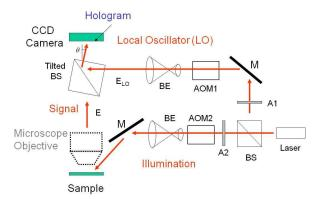
Fig. 1. Digital holography setup. AOM1 and AOM2 : acousto-optic modulators; BS : beam splitter; BE : beam expander; M : mirror; A1 and A2 : attenuator;  $\theta$  : tilt angle of the beam splitter with respect to optical axis
