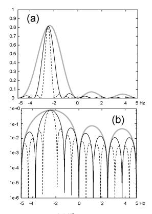
Fig. 3. Frequency response  $|\eta(x)|^2$  for heterodyne signal in intensity, as a function of the heterodyne beat frequency  $x = f - f_{LO}$  for sequences of 4n frames with 4n = 4 (heavy grey line), 4n = 8 (solid black line), and 4n = 16 (dashed black line). Calculation is done for T = 0.1 s. Vertical axis axis is  $|\eta(x)|^2$  in linear (a) and logarithmic (b) scales. Horizontal axis is  $x = f - f_{LO}$  in Hz.
