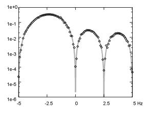
Fig. 4. Frequency response for heterodyne signal in intensity, as a function of the heterodyne beat frequency  $x = f - f_{LO}$  for a sequence of 4 frames: theory  $|\eta(x)|^2$  (heavy grey line), and experiment W(x) (points). Calculation and experiment are done with T = 0.1 s. Vertical axis axis is  $|\eta(x)|^2$  or W(x) in logarithmic scales. Horizontal axis is  $x = f - f_{LO}$  in Hz.
