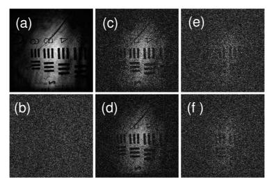
**Fig. 4** (a,c,d): Reconstructions of an USAF target with different level of illumination 700 (a), 1 (c) and 0.15 e/pixel (d). (b): Simulated Shot Noise noise image. (e,f): Simulated reconstructed image obtained by mixing image (a) with weight X, and image (b) with weight 1-X. The weight X is 1/700 (e), and 0.15/700 (f). Images are displayed in arbitrary logarithmic grey scale.
