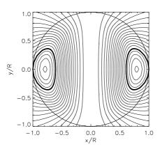
Figure 1. The field lines of a twisted-torus magnetic field configuration, projected in the meridional plane. The toroidal field is confined in the region inside the thick curves.
