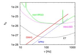
Figure 2. Gravitational signal emitted by a rotating NS at a distance of 10 kpc, deformed by a twisted-torus magnetic field, with  $B_{pole} = 10^{15}$  G,  $\alpha = 3^{o}$ ,  $M = 1.4 M_{\odot}$  and EOS GNH3 (solid line) and APR2 (dotted line). The sensitivity curves of advanced LIGO, advanced VIRGO (with integration time of three months) and ET (with integration time of one year) are shown for comparison.
