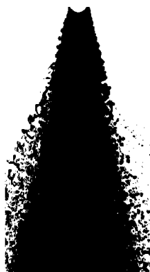
Figure 7 : Superposition of the successive positions of the jet, for U_g = 14 m/s and U_l = 0.28 m/s.
