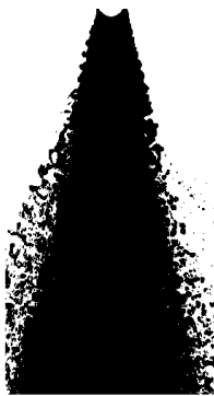
Figure 7 : Superposition of the successive positions of the jet, for U_g = 14 m/s and UI = 0.28 m/s.
