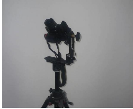
Figure 11: Camera set on the panoramic heading
