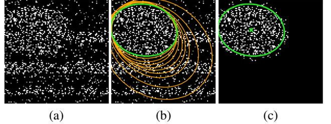
**Fig. 2.** (a) Original 2D synthetic image, corrupted by salt-and-pepper noise. (b) Evolution of the ellipsoid. (c) Ellipse contour and center superimposed on the weighting function  $wI$  at convergence.
