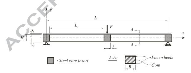
Fig. 8: Sandwich beam specimen. L = 300 mm,  $L_1 = 130$  mm,  $L_{ins} = 20$  mm, B = 30 mm,  $H_c = 20$  mm,  $t_f = 1$  mm
