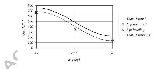
Fig. 11: Comparison of apparent shear modulus  $G_{xy}(\alpha)$  found by: laminate theory with material properties estimated according to [8], lap shear test, sandwich beam 3-point
