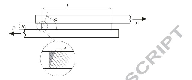
Fig. 6: Determination of length detriment according to the specimen grain direction, where the shaded area d is ignored for the purpose of assessing the shear stiffness  $G_{xy}$ .
