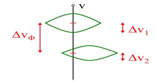
FIG. 6: Snapshot of the trapping domains of two nearby waves. They have half-widths  $\Delta v_i$  and a mismatch in velocity  $\Delta v_{\Phi}$ .
