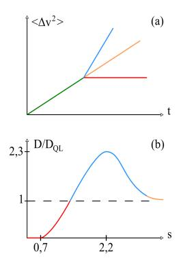
Fig. 7 Regimes of diffusion. (a)  $\langle \Delta v^2 \rangle$  vs. time; initial quasilinear regime: green line; asymptotic saturation: red line; superquasilinear regime: blue line; time-asymptotic quasilinear regime: brown line. (b)  $D/D_{\text{QL}}$  vs. *s*; same color code as in (a), except for the red growing segment that corresponds to the weakly chaotic regime.
