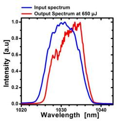
Figure 4: (Color online) Optical spectrum measured (blue) at the output of the frontend and (red) after compression at maximum energy.
