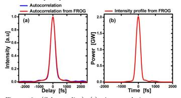
Figure 3: (Color online) (a) Autocorrelation traces measured at 650  $\mu$ J (blue) with an independent autocorrelator and (red) from a FROG measurement. (b) Retrieved temporal profile of the pulse from the FROG measurement (Error 27.10<sup>-4</sup> on a 256 x 256 grid).
