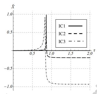
Figure 5. Coordinate,  $\hat{X}$ , of the contact point for initial conditions IC1, IC2 and IC3. Notice that for rocking (IC1) the  $X_P$  coordinate of the drum remains constant (zero), while for IC2 and IC3 is not. This means that the contact point is not limited in the plane of the two dimensional rocking motion.
