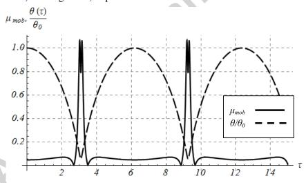
Figure 3. Mobilized friction coefficient and normalized inclination angle of the column presented in Figure 4. The energy dissipated during the short time intervals of sliding (peaks of the mobilized friction coefficient) generally results to a practically smooth collisionless contact.
