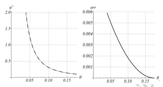
Figure 7. On the left  $\varphi'$  versus  $\theta$  is plotted for a) the numerical solution (solid line) and b) the approximation of Eqs.(26) (dashed line). On the right the relative error of the approximation is presented, which is less than 6‰.
