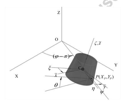
Figure 2. Coordinate systems and Euler angles. O(X,Y,Z) is the inertial frame,  $P(X_P,Y_P)$  the contact point with the horizontal plane,  $\theta$  the inclination angle,  $\varphi$  the precession angle and  $\psi$  the rotation about  $\zeta$ -axis.
