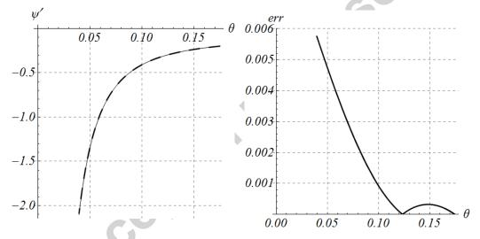
Figure 8. On the left  $\psi'$  versus  $\theta$  is plotted for a) the numerical solution (solid line) and b) the approximation of Eqs.(26) (dashed line). On the right the relative error of the approximation is presented, which is less than 6‰.
