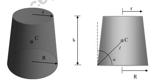
Figure 1. The conical frustum: 3D and 2D view.
