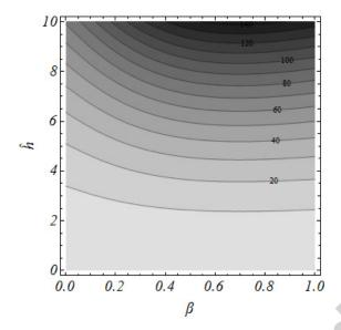
Figure 9. Contour plot of  $ps(\hat{h}, \beta)$  as function of the slenderness  $\hat{h}$  and the conicity  $\beta$  of the conical frustum.
