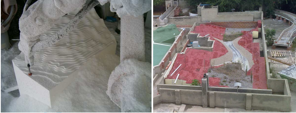
Figure 15. Left, milling process of an EPS block; right, final 1:75 model used for flowing simulation (real dimensions of 8x13 m).
