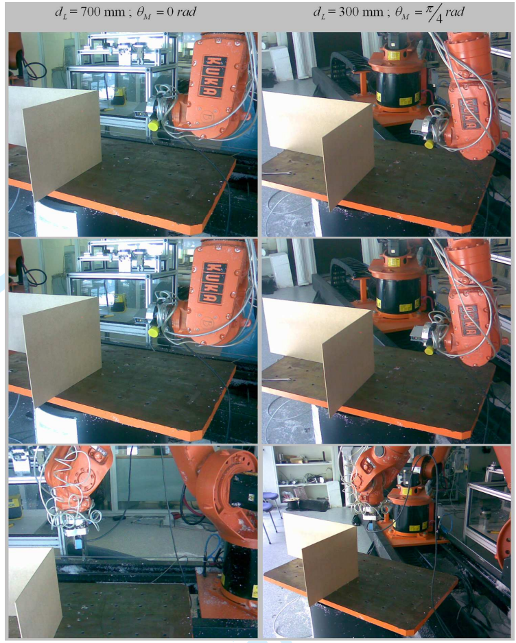
Figure 7. Sweeping the reference planes with two configurations of d_L and \theta_M .
