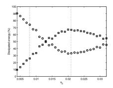
**Fig. 2.** Percentage of energy dissipated by the linear chain (circle markers) and by the NES (square markers) versus level excitation  $s_0$ .
