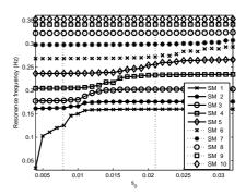
**Fig. 3.** SD of the system with NES: resonance frequencies estimated from SD versus level excitation  $s_0$ .
