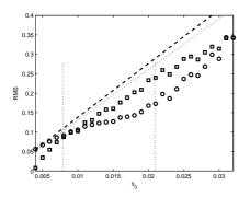
**Fig. 1.** *RMS chain* for the system with the NES (circle markers), with only the linear part of the NES (dotted line), without NES (dashed line) and *RMS NES* (square markers) versus level excitation  $s_0$ .
