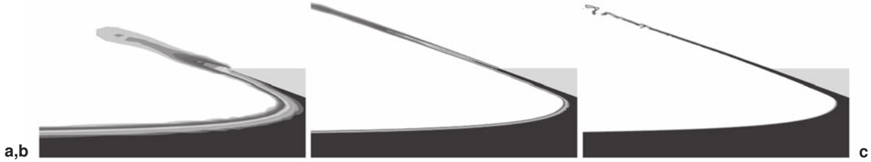
Fig. 13. Influence of NGen on the free-surface definition. a NGen = 1. b NGen = 3. c NGen = 5
