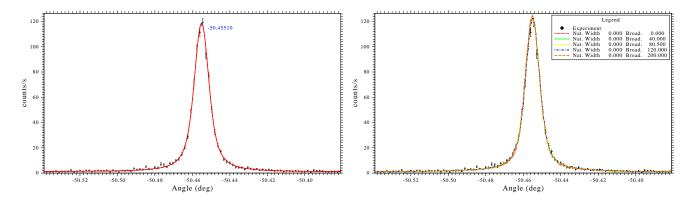
Figure 13. (Color online) Voigt profile (left) and simulated profiles with different line width (right) fitted to an experimental non-dispersive mode spectrum. The Voigt profile fit yield a  $\chi^2 = 1.12$  while the simulated ones gives  $\chi^2$  ranging from 1.2 to 1.4 (the variation is mostly due to the statistic of the simulated profiles). The difference in angle is equal to  $1.3 \times 10^{-4}$  Degrees.
