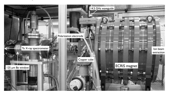
Figure 3. The SIMPA ECRIS and its connexion to the spectrometer
