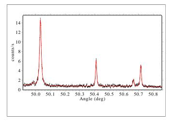
Figure 22. (color online) Experimental survey dispersive spectrum. Left peak:  $1s^22s^22p^1P_1 \rightarrow 1s^22s^2{}^1S_0$  in  $\mathrm{Ar}^{14+}$ , central peak:  $1s2s^3S_1 \rightarrow 1s^2{}^1S_0$  in  $\mathrm{Ar}^{16+}$ , left peaks:  $1s2s2p^2P_{1/2,\,3/2} \rightarrow 1s^22s^2S_{1/2}$  in  $\mathrm{Ar}^{15+}$ . The line represents a fit using a sum of Voigt profiles.
