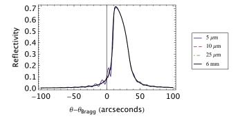
Figure 21. (Color online) Reflectivity curves for different crystal thicknesses evaluated with XOP. Only the  $5~\mu m$  and the  $10~\mu m$  profiles shows pendellosung oscillations.
