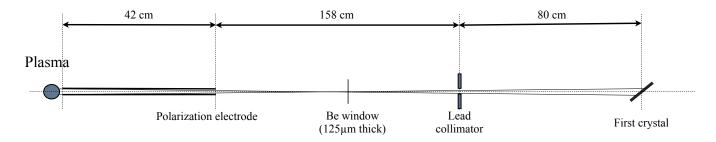
Figure 2. Geometrical arrangement of the DCS, polarization electrode, lead collimator and of the SIMPA ECRIS plasma. The inner diameter of the polarization electrode is 12 mm.
