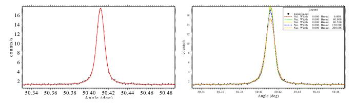
Figure 14. (Color online) Voigt profile (left) and simulated profiles with different line widths (right) fitted to an experimental dispersive mode spectrum. The Voigt profile fit yield a  $\chi^2=1.42$  and the optimum simulated profile one (for a Gaussian broadening of 80 meV) gives a  $\chi^2=1.26$ . The difference in angle between the peak position between the two fits is equal to  $1.86(7) \times 10^{-3}$  Degrees.
