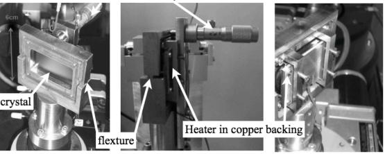
Figure 8. Details of the crystal support, with the vertical tilting system (composed of a flexture and of a micrometric screw) and the heater plate for temperature control. The copper plate ensures uniform repartition of heat on the back of the crystal. A graphite foil is positioned between the crystal and the copper plates to improve thermal contact under vacuum.
