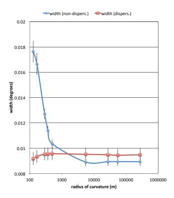
Figure 18. (Color online)Widths of the dispersive and nondispersive profiles as a function of the crystals radius of curvature. These width are obtained by fitting simulated spectra with a Voigt profile and combining the Lorentzian and Gaussian widths using Eq. (20). Error bars are du to statistic. The dispersive and non-dispersive widths are identical for large radii of curvature as expected, within simulation statistical uncertainty.
