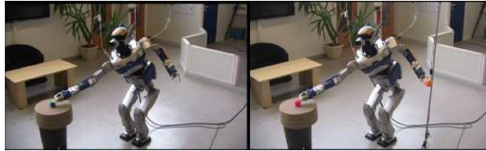
Scenario (c): To grasp the ball in front of it (left), the robot reaches a posture where the left arm is used to maintain its balance. In the figure on the right, the robot performs two actions in parallel: grasping a ball in front of it while grasping a ball behind (of course the ball behind has been intentionally placed at the end position of the left hand depicted on the left side). It is not possible to spot the difference between both postures. However, the question we address is: Is it possible to spot the difference between both motions ?
