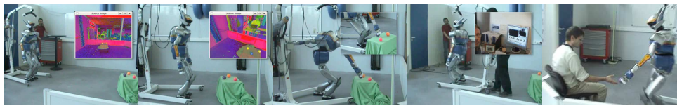
Scenario (a): The global task Give me the ball is decomposed into a sequence of sub-tasks [locate the ball], [walk to the ball], [grasp the ball], [locate the operator], [walk to the operator], and [give the ball]. The motions [walk to], [grasp], [give] appear as a sequence structuring the action (from [2]).
