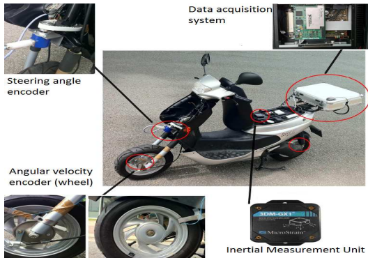
Fig. 7. Sensors implementation on our Motorcycle
