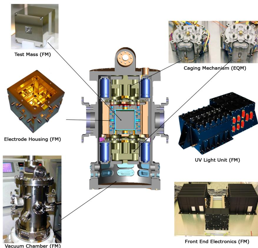
**Figure 2.** Photographs of the Inertial Sensor Subsystem flight models (FM) and engineering qualification models (EQM). From bottom left: Vacuum Chamber (Carlo Gavazzi Space), Electrode Housing (Thales Alenia Space), (uncoated) Test Mass (Thales Alenia Space), Caging Mechanism (Thales Alenia Space), UV Lamp Unit (Imperial College London), Front-End Electronics (ETH, Zurich).
