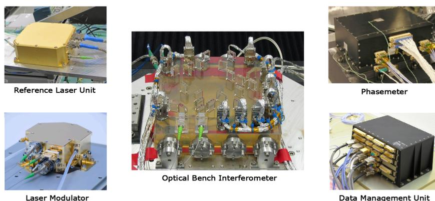
**Figure 3.** Photographs of the Optical Metrology System Flight Hardware. From top left: Reference Laser Unit (Tesat), Phasemeter (Uni Birmingham), Data Management Unit (ICE, Barcelona), Laser Modulator (APC/Contraves). Centre: Optical Bench Interferometer (Uni Glasgow)
