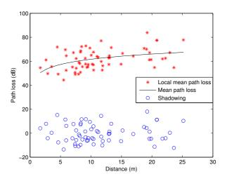
Fig. 6. The obtained local mean path loss, mean path loss and shadowing from measurement.
