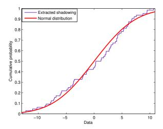
Fig. 4. CDF comparison between the extracted shadow fading from the MR-FDPF method and normal distribution.
