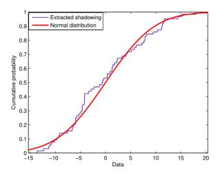
Fig. 7. CDF comparison of the extracted shadowing and normal distribution from measurement.
