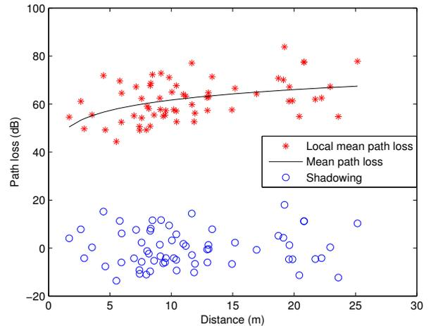
Fig. 6. The obtained local mean path loss, mean path loss and shadowing from measurement.
