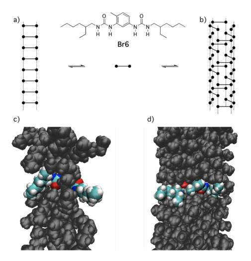
**Figure 1.** Schematic representations (a and b) and optimized geometries<sup>14b</sup> (c and d) for bis-urea **Br6** in filament (a and c) or tube (b and d) forms. In each assembly, a single bis-urea is highlighted with O in red, N in blue, C in light blue and H in white.
