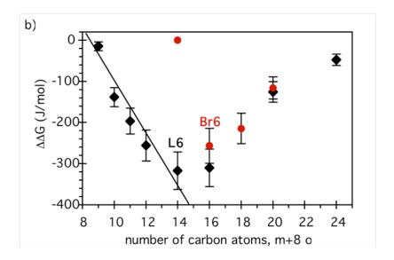
**Figure 2.** (a) Transition temperature for bis-ureas **Br5** to **Br8** (red) and bis-urea **L1** to **L16** (black), measured in toluene (10mM). (b) Relative free energy of the tube to filament transition, versus alkyl chain length (the reference is **Br5** and the reference temperature is 27.4°C).
