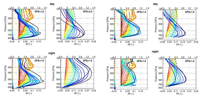
**Fig. 2.** SOFRID (left panel) and FORLI (right panel) averaging kernels (AK) (bottom x-axis, colour lines) and normalised averaging kernels of partial columns (top x-axis, black solid line: surface–480 hPa, black dashed line: 480–225 hPa), for a daytime (top panels) and nighttime (bottom panels) retrieval of a IASI pixel near Frankfurt (50.1° N, 8.7° E) on 28 May 2008. The nominal height of each averaging kernel is marked by the horizontal tick with corresponding colour.
