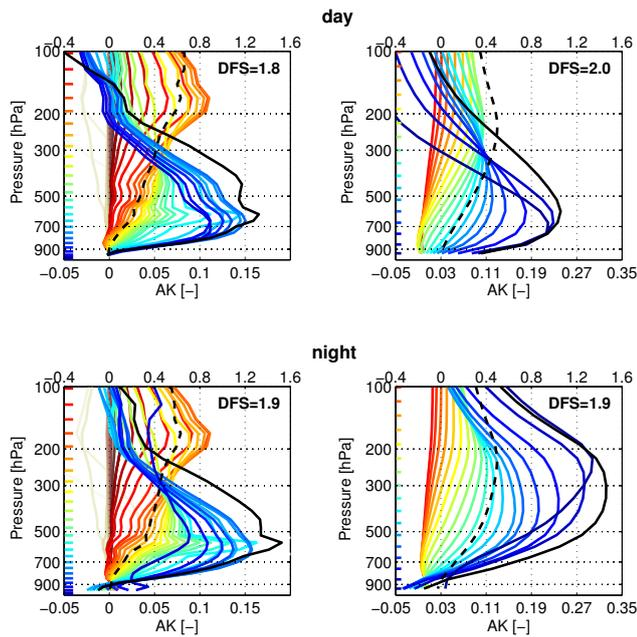
**Fig. 2.** SOFRID (left panel) and FORLI (right panel) averaging kernels (AK) (bottom x-axis, colour lines) and normalised averaging kernels of partial columns (top x-axis, black solid line: surface–480 hPa, black dashed line: 480–225 hPa), for a daytime (top panels) and nighttime (bottom panels) retrieval of a IASI pixel near Frankfurt (50.1° N, 8.7° E) on 28 May 2008. The nominal height of each averaging kernel is marked by the horizontal tick with corresponding colour.
