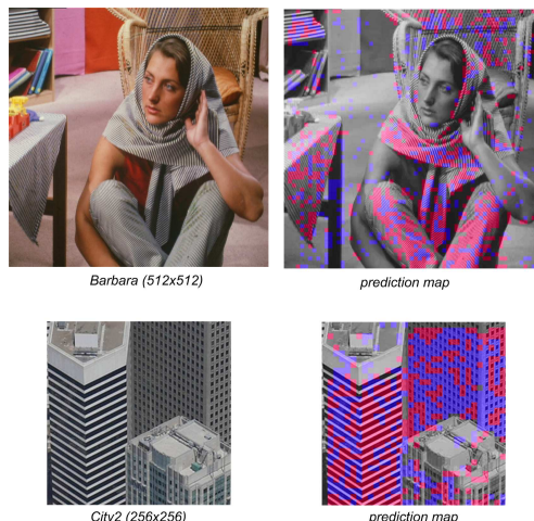
Fig. 4. Illustration of modes used in 8x8 prediction: TM (in blue) and BM (in red) (QP=31).
