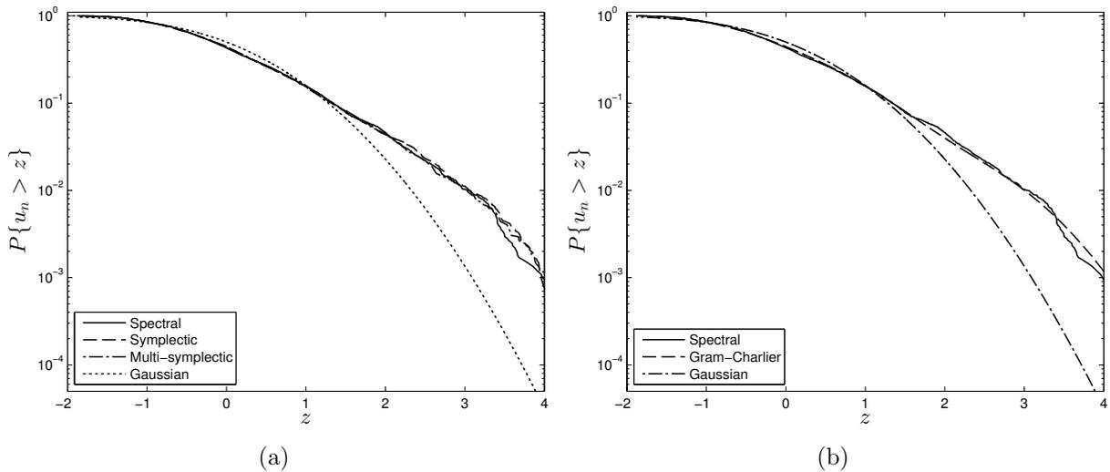
FIGURE 14. Random wave field: (a) probability of exceedance of the normalized wave surface  $u_n$  predicted by the numerical schemes, and (b) observed statistics against Gaussian and Gram-Charlier distributions.
