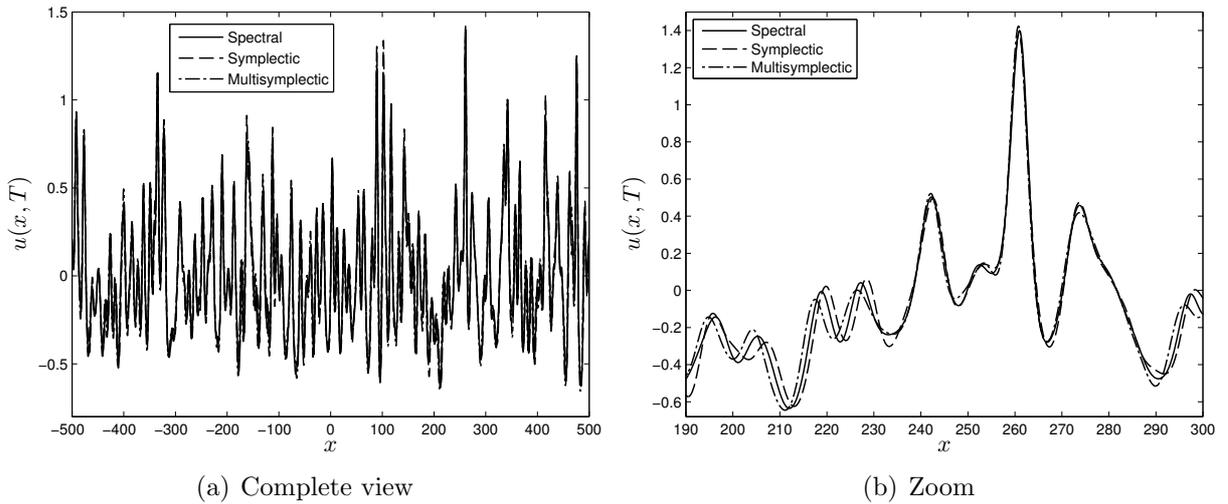
FIGURE 10. Random wave field: Comparison of numerical solutions at final time  $T = 800$  computed by the spectral, symplectic and multi-symplectic schemes. The right image (b) shows a zoom on the segment  $190 \leq x \leq 300$ .
