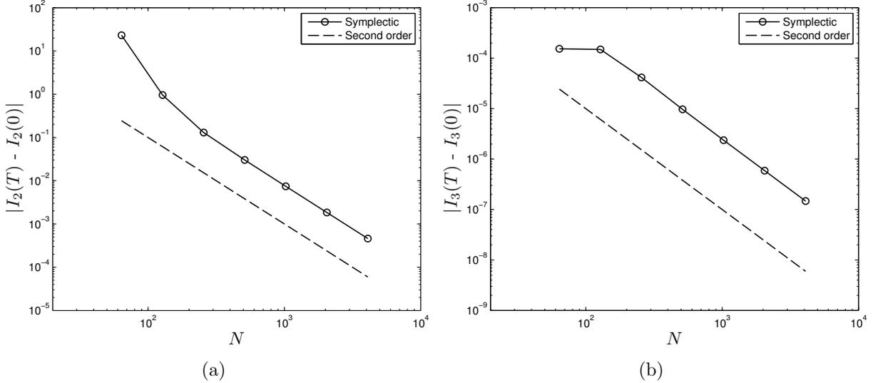
FIGURE 3. Test-case B (two-soliton collision): conservation of the invariants  $\mathcal{I}_2$  and  $\mathcal{I}_3$  as function of the grid size  $N$  for the symplectic scheme (2.4): the second order convergence rate.
