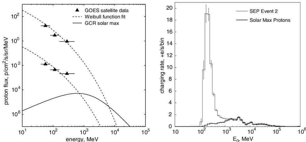
**Figure 5.** Left panel: spectra of primary energies in a giant SEP event (September 1989) and of a normal one (May 2001) as obtained from the GOES Observatory data, and fitted. Also shown is a GCR proton spectrum taken at solar maximum. Right panel: charging rates in the TMs for a “normal” SEP event and GCR, also at solar maximum.
