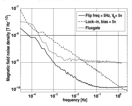
**Figure 4.** Magnetometers sensitivity curves. The horizontal, thicker grey line at  $10^{-8}~{\rm Tesla\,Hz^{-1/2}}$  is the current LPF magnetometer noise requirement, which is comfortably met in all cases considered, i.e., for frequencies above 1 mHz. The curves show that the best performance corresponds to the AMR with a *flip* voltage scheme, showing significant improvements over the more conservative lock-in approach. The Fluxgate performs well but is slightly noisier at LISA frequencies.
