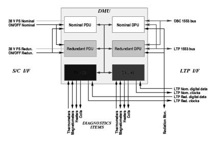
Figure 7. Schematics of the DMU boards and their LTP interfaces.
