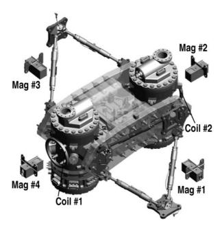
**Figure 3.** LTP diagnostic magnetometers and induction coils. For clarity, the former are shown levitating, but they are actually bolted to the surrounding cylindrical wall with the shown braces.
