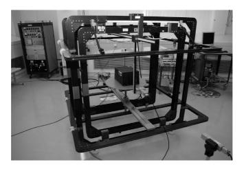
${\bf Figure~8.~} {\bf The~DMU~} {\rm in~a~test~facility~at~ESTEC.~} {\bf It~is~the~dark~box~at~the~centre~} {\rm of~a~Helmholtz~coil~set,~which~shields~the~DMU~} {\rm from~external~disturbances~during~magnetic~moment~measurements.}$
