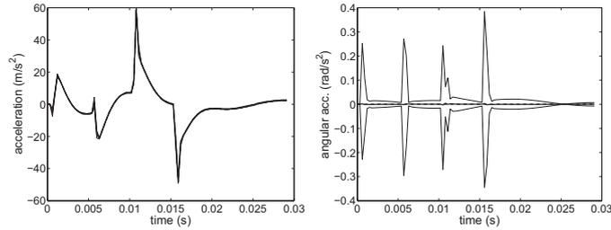
Figure 3: Random transient acceleration of point  $P_{obs}$ , Case 2: confidence region (upper and lower envelopes), mean response and response of the mean model are superimposed;  $x_{0,3}$ -acceleration (left figure) and  $x_{0,1}$ -angular acceleration (right figure).
