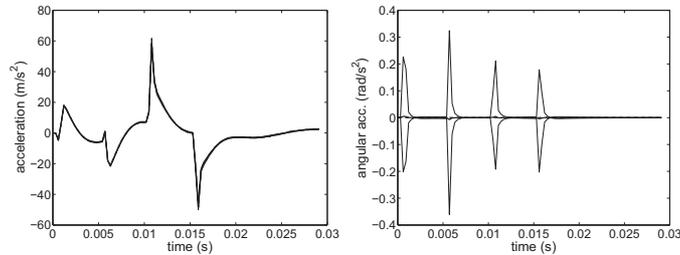
Figure 4: Random transient acceleration of point  $P_{obs}$ , Case 3: confidence region (upper and lower envelopes), mean response and response of the mean model are superimposed;  $x_{0,3}$ -acceleration (left figure) and  $x_{0,1}$ -angular acceleration (right figure).
