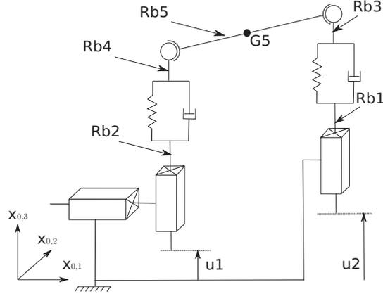
Figure 1: Rigid multibody system.
