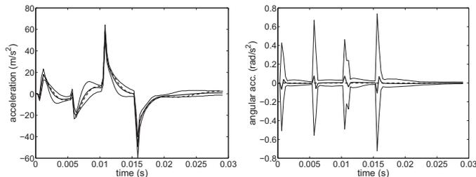
Figure 5: Random transient acceleration of point  $P_{obs}$ , Case 4: confidence region (upper and lower thin solid lines), mean response (thick solid line) and response of the mean model (dashed line);  $x_{0,3}$ -acceleration (left figure) and  $x_{0,1}$ -angular acceleration (right figure).
