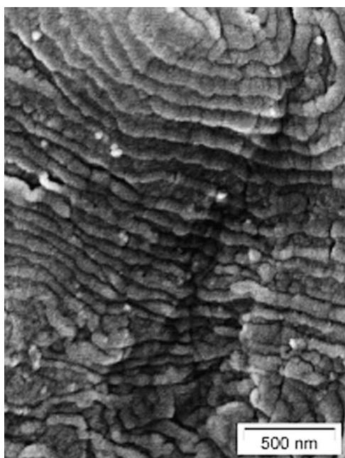
FIGURE 5 SEM micrograph of the PS 272 PAPTES 130 PS 268 hybrid film after calcination at 800 °C.
