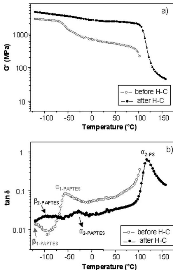
**FIGURE 6** Temperature dependence at 5 Hz of (a)  $G'$  and (b)  $\tan \delta$  for the PS<sub>272</sub>PAPTES<sub>130</sub>PS<sub>268</sub> copolymer before and after the hydrolysis-condensation (H-C).
