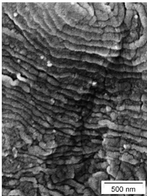
**FIGURE 5** SEM micrograph of the PS<sub>272</sub>PAPTES<sub>130</sub>PS<sub>268</sub> hybrid film after calcination at 800 °C.
