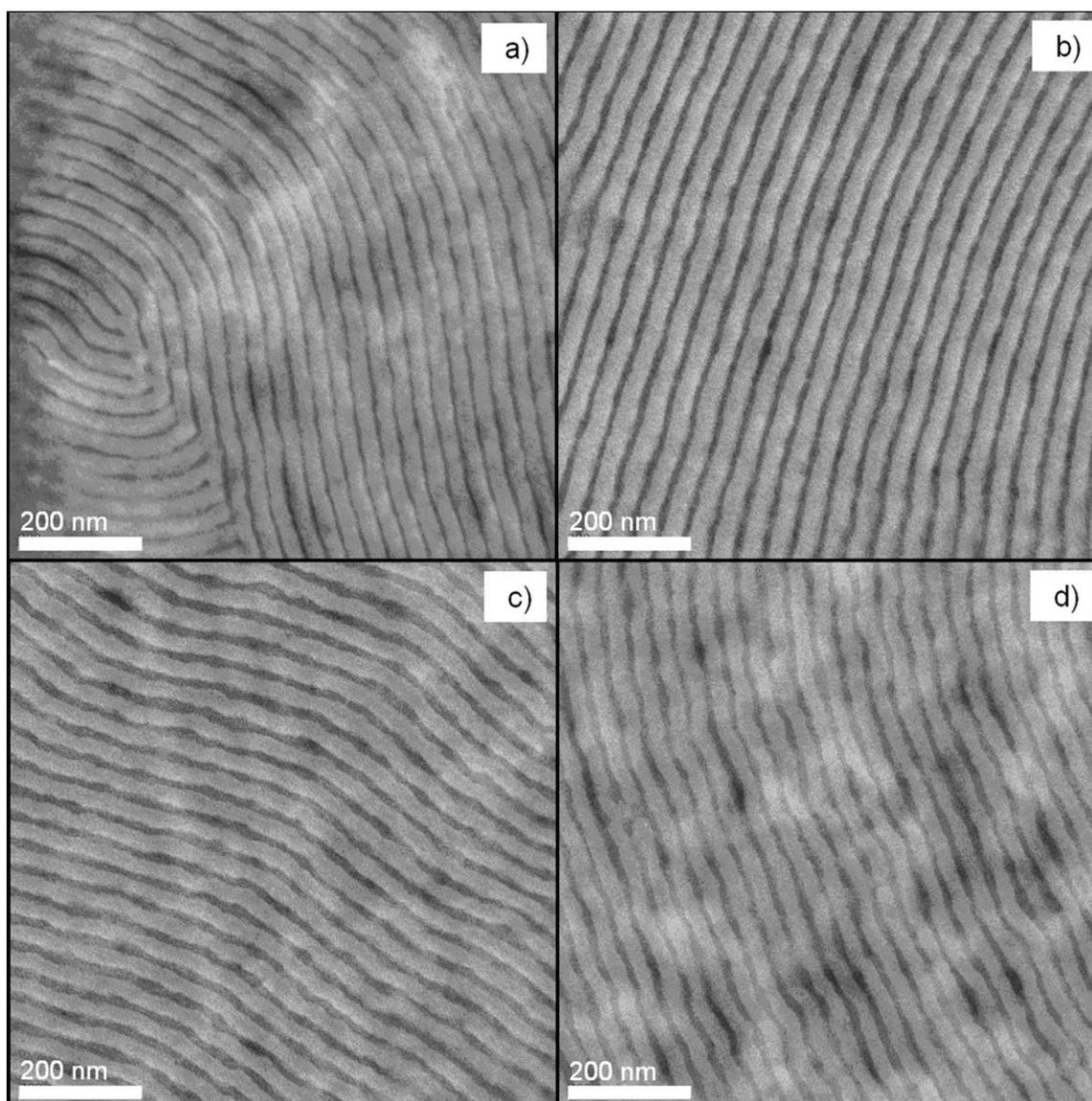
**FIGURE 2** TEM micrographs of the PS-*b*-PAPTES-*b*-PS triblock copolymer self-assembled thin films: (a) PS<sub>272</sub>PAPTES<sub>130</sub>PS<sub>268</sub>, (b) PS<sub>272</sub>PAPTES<sub>224</sub>PS<sub>260</sub>, (c) PS<sub>272</sub>PAPTES<sub>290</sub>PS<sub>293</sub>, and (d) PS<sub>272</sub>PAPTES<sub>336</sub>PS<sub>269</sub> (annealed at 150 °C for 72 h).
