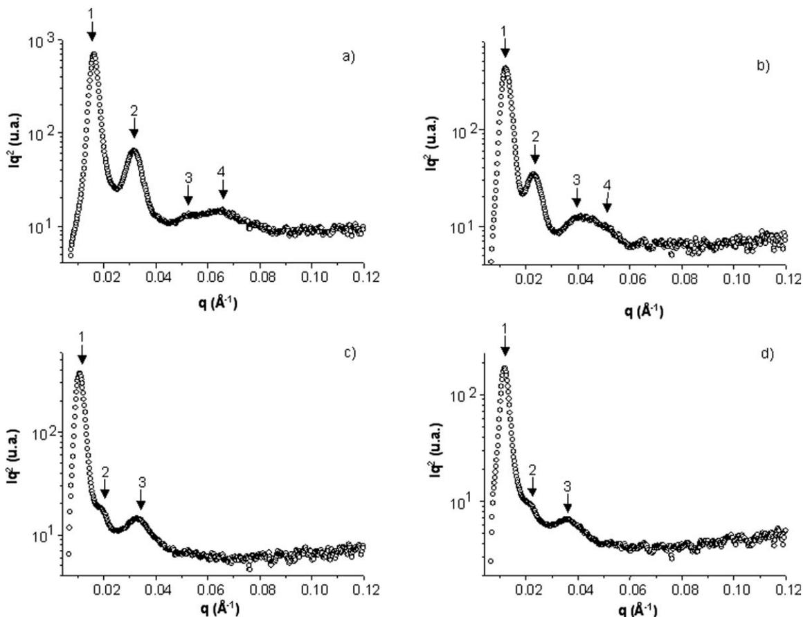
**FIGURE 3** SAXS curves of the films obtained from the different copolymers: (a) PS<sub>272</sub>PAPTES<sub>130</sub>PS<sub>268</sub>, (b) PS<sub>272</sub>PAPTES<sub>224</sub>PS<sub>260</sub>, (c) PS<sub>272</sub>PAPTES<sub>290</sub>PS<sub>293</sub>, and (d) PS<sub>272</sub>PAPTES<sub>336</sub>PS<sub>269</sub> after annealing at 150 °C for 72 h.
