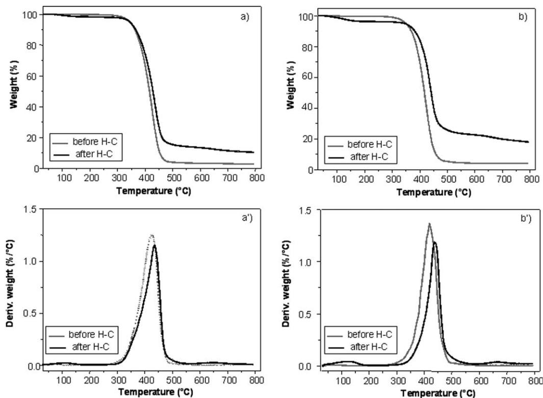
**FIGURE 4** TGA curves of (a) PS<sub>272</sub>PAPTES<sub>130</sub>PS<sub>268</sub> and (b) PS<sub>272</sub>PAPTES<sub>290</sub>PS<sub>293</sub> before and after the hydrolysis–condensation (H-C) and their associated first derivatives (a' and b').
