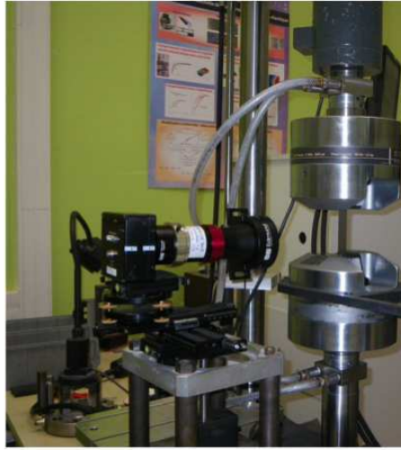
Figure 2: Test configuration for the cyclic loading. A telecentric lens is used to minimize artifacts induced by out-of-plane motions.
