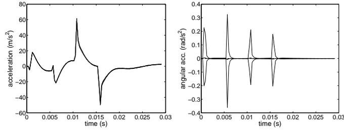
Figure 5: Random transient acceleration of point  $P_{obs}$ , Case 3: confidence region (upper and lower envelopes), mean response and response of the mean model are superimposed;  $x_{0,3}$ -acceleration (left figure) and  $x_{0,1}$ -angular acceleration (right figure).
