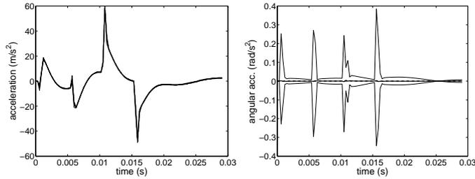
Figure 4: Random transient acceleration of point  $P_{obs}$ , Case 2: confidence region (upper and lower envelopes), mean response and response of the mean model are superimposed;  $x_{0,3}$ -acceleration (left figure) and  $x_{0,1}$ -angular acceleration (right figure).
