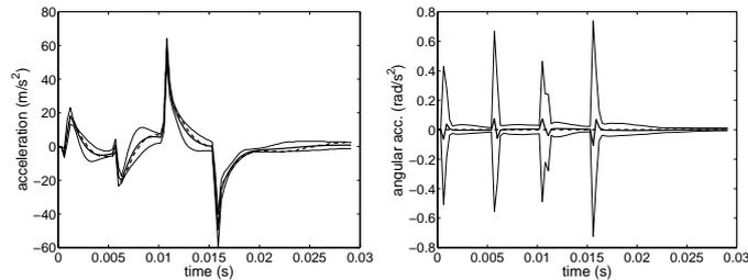
Figure 6: Random transient acceleration of point  $P_{obs}$ , Case 4: confidence region (upper and lower thin solid lines), mean response (thick solid line) and response of the mean model (dashed line);  $x_{0,3}$ -acceleration (left figure) and  $x_{0,1}$ -angular acceleration (right figure).
