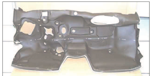
Figure 1: Picture of a sound-insulation device (dash trim)
