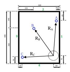
Fig. 2 Experimental configuration (distances in millimetres),  $R_A = 241$ ,  $R_B = 251$ ,  $R_C = 235$
