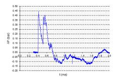
**Fig. 39**Pressure-time history - Sensor C - Walls 1 + 2
