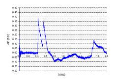
Fig. 41Pressure-time history - Sensor C - Walls 1 + 4
