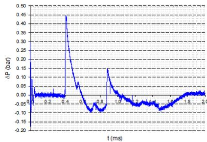
**Fig. 22** Pressure-time history - Sensor B - Wall 3 alone
