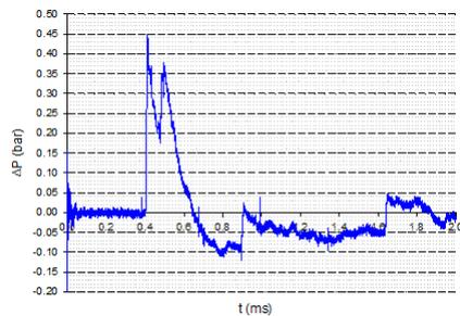
**Fig. 43** Pressure-time history - Sensor C - Walls 2 + 4
