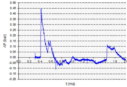
**Fig. 39** Pressure-time history - Sensor C - Walls 1 + 2
