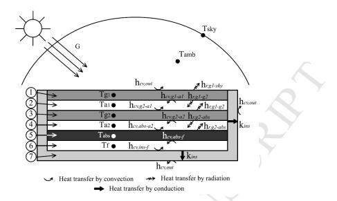
Fig. 2: Representation of the double glazed collector: 1. First glass layer 2. First air layer 3. Second glass layer 4. Second air layer 5. Absorbent surface 6. Transfer fluid 7. Insulation and support.
