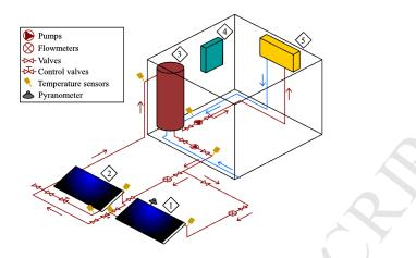
Fig. 3: Test bench schematic: 1. Collector N<sup>•</sup>1, 2. Collector N<sup>•</sup>2, 3. Storage tank, 4. Control device, 5. Fan coil.
