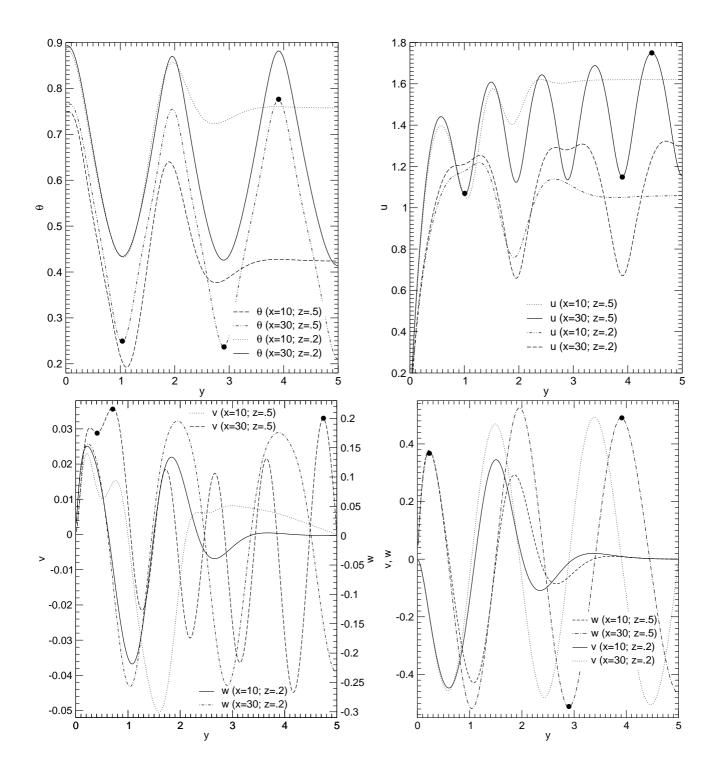
Figure 4: Spanwise profiles of the primitive variables  $\theta$ , u, v and w obtained by the four contributors along the lines at (x, z) = (10, 0.2), (10, 0.5), (30, 0.2) and (30, 0.5). The filled circles indicates the local extrema whose values and coordinates are given in Table 3.
